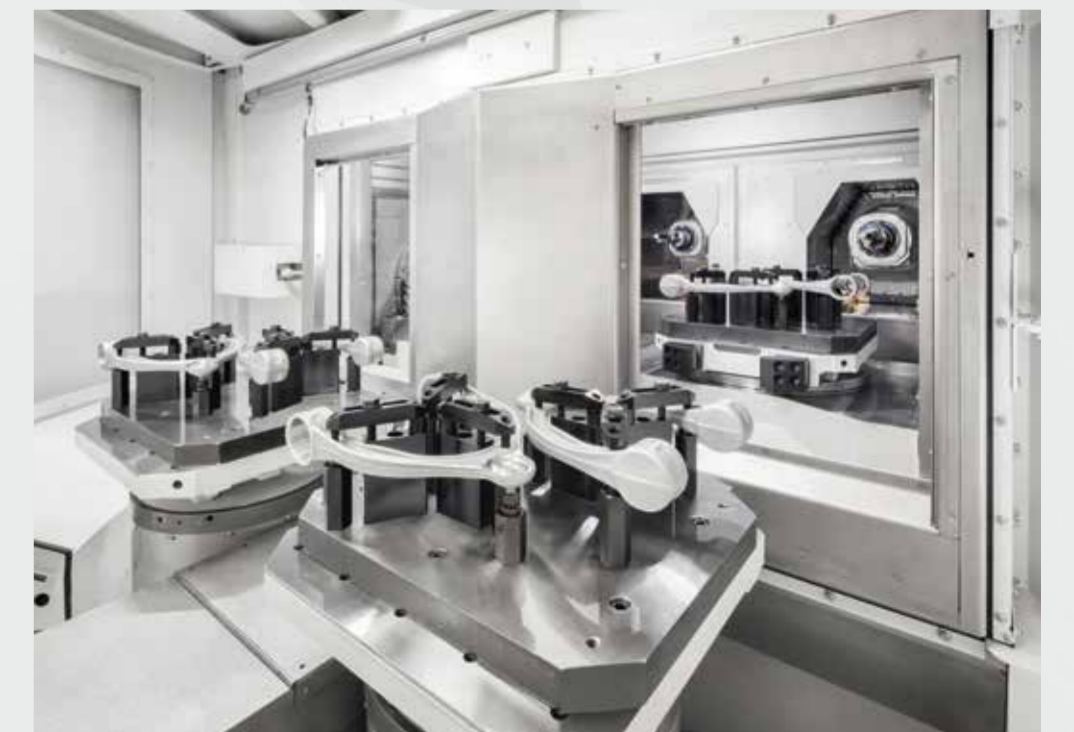
Machining of suspension arms on a double-spindle G-module
