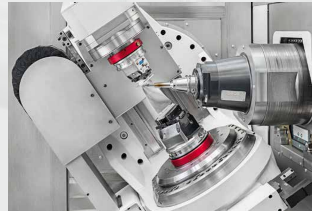
VARIO rotary table with steady rest and tandem drive
