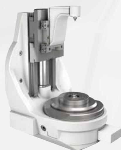
Steady rest with tailstock center
